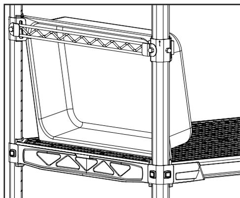
**Note:** Accessory Rail (XHR24S) is mounted to two add-a-collars that are installed 4 positions above the shelf.
