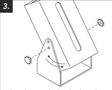
Adjust dispenser box to the desired angle, insert and tighten the Pivot Pin (4)
